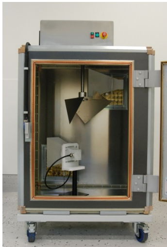
Figure 1. Photograph showing the reverberating chamber (RC) with transmit and receive antennas. The chamber internal volume is 1.24 \times 0.98 \times 0.82 \text{ m}^3 and the lowest usable frequency (LUF) is 1 GHz.
