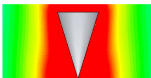
Fig.6 Radiation field distribution characteristic of upright conic monopole
