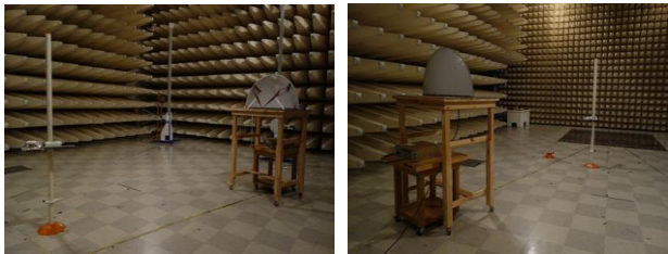
Figure 5. Measurement setup in a semi-anechoic room
