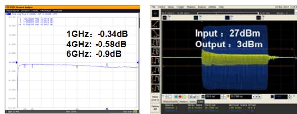
Figure 7. Test results of the passive limiter circuit based on dice-packaged PIN diodes. Left, S21 (Vertical, insertion loss, 2 dB/div; horizontal, frequency, 800 MHz/div). Right, input and output signals (Blue lines, input signal; yellow lines, output signal. Vertical, voltage, V; horizontal, time, 20 ns/div).
