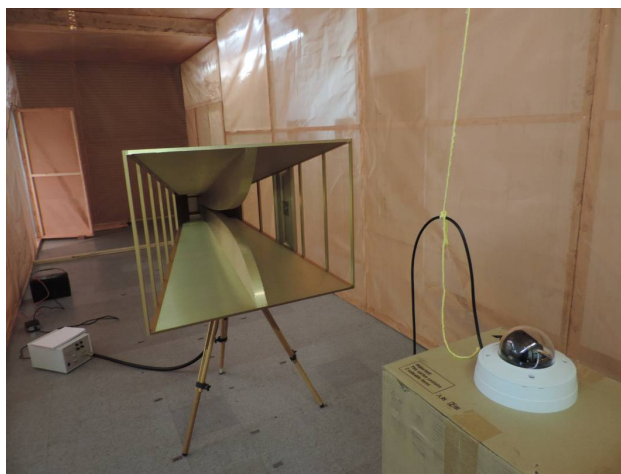
Figure 1. Photo of one of the radiated tests. (Here the cable is looped to increase exposure.)
