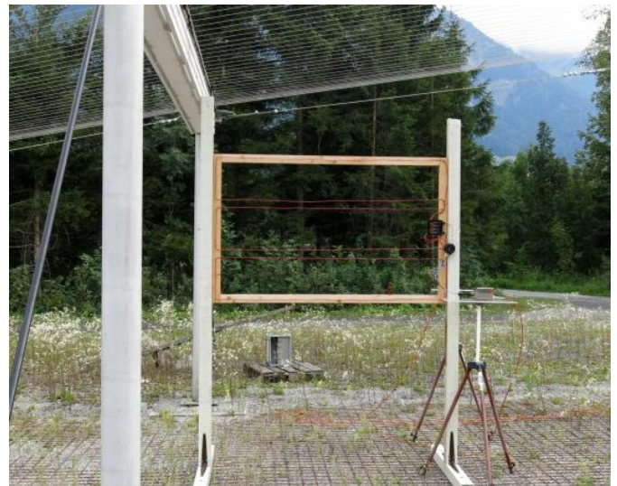
Figure 4: Wire model of a PV-module with 3x20 arrays and junction box for studying and measuring the HEMP-coupled currents
